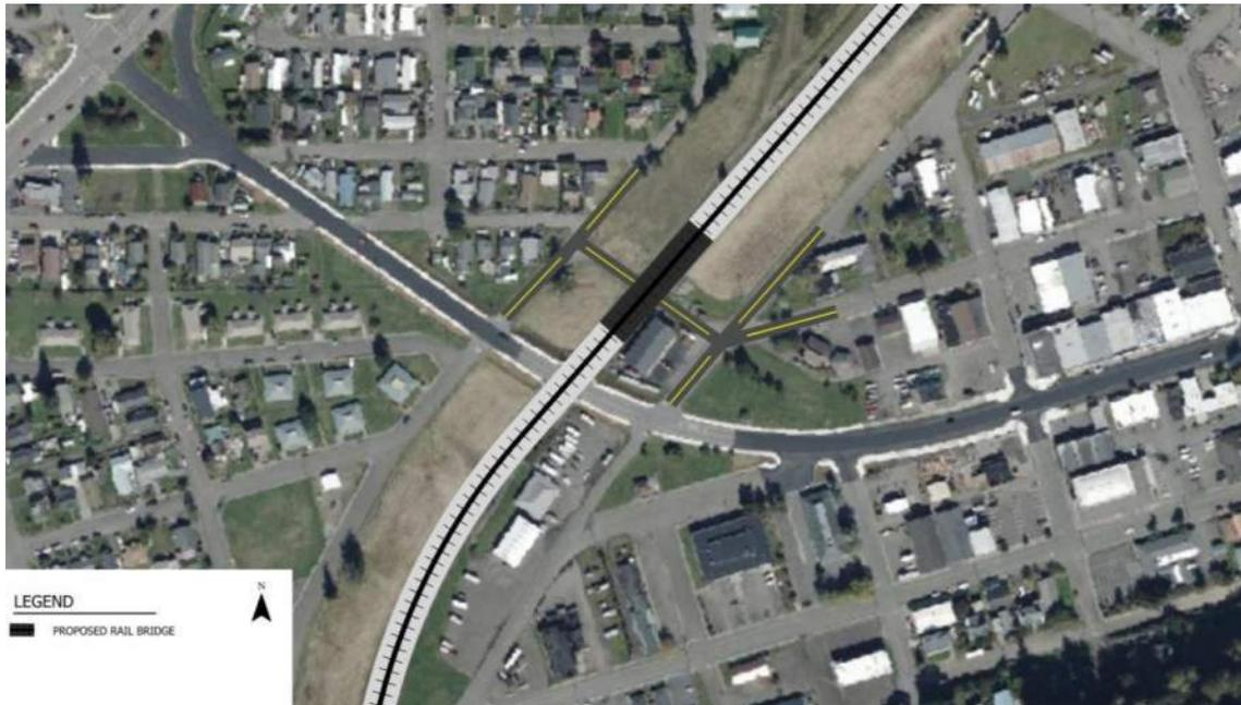
**Planning level cost opinion:** An order-of-magnitude planning level cost opinion was prepared for the northerly OR 38 undercrossing upgrades based on unit costs from similar projects in the Pacific Northwest. The cost opinion accounts for design and construction along with several other factors. Potential right-of-way and property costs are not included at this time. The cost opinion is \$7.0M.
