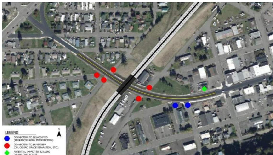
**Planning level cost opinion:** An order-of-magnitude planning level cost opinion was prepared for the OR 38 rail undercrossing with retaining walls based on unit costs from similar projects in the Pacific Northwest. The cost opinion accounts for design and construction along with several other factors. Potential right-of-way and property costs are not included at this time. The cost opinion is \$13.0M.
